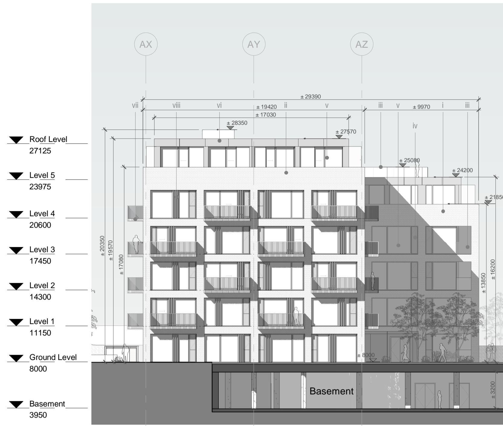
1 Building A - South Elevation scale 1 : 200
